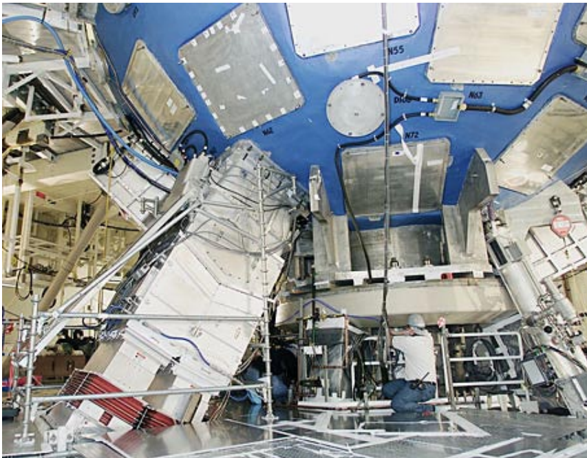
Quad 31b beamtubes and optics are installed and operational
